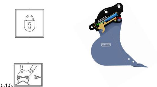
With the bucket placed on the ground, visually check that the coupler is fully engaged and safely locked to the bucket.
