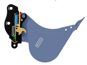
**5.2.2.** Slowly roll the coupler backwards, away from the cab, and the bucket will disengage from the rear pin before placing the bucket onto the ground.
